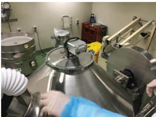
Figure 1: Interface of the MicroNIR PAT-W into the lid of a double cone blender.
