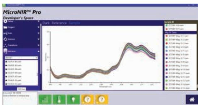
Figure 2: Raw NIR spectra obtained for a blend uniformity analysis.
