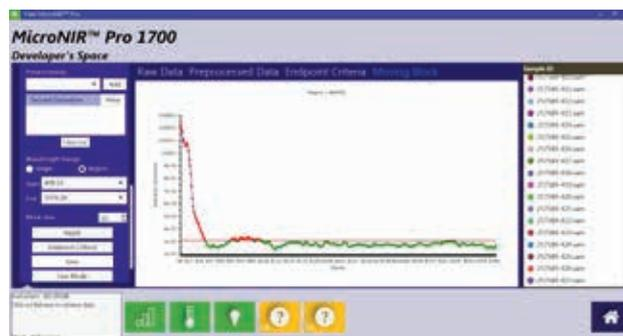
Figure 3: Moving Block Standard Deviation (MBSD) Chart for blend uniformity analysis.
