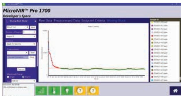
Figure 5: Monitoring lubricant blending using MicroNIR PAT-W
