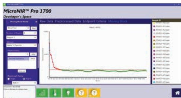
Figure 4: Application of the Moving Block Standard Deviation (MBSD) model to a validation batch.
