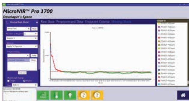
Figure 6: Application of lubrication blend model to a validation batch
